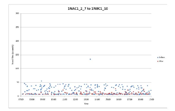
The average after delay has been reduced to near 'zero'. It was noted that any trams that did occur delay were trams with headways to the previous tram of less ten the travel time from the initiating strategy detector at Glossop Road. Hence these trams overlapped with a tram already being given the strategy and STM was unable to begin the optimization until the previous tram had cleared Shalesmoor.
